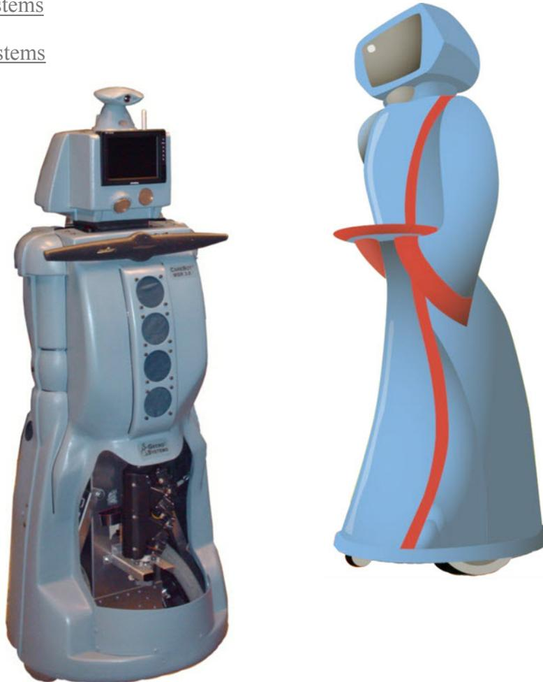
The 2005 CareBot™ with our Compound Sensor Array™ along with a 2012 concept drawing of slimmed down, simplified design which has become possible with the advent of the depth camera and other improved technology.
